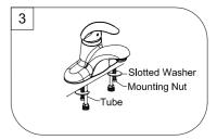
Insert supply TUBES through holes of sink . Attach SLOTTED WASHERs and hand tighten MOUNTING NUTs .
