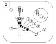
2. Unscrew the nut (5) and washer (4) from the pipe body (7), retain the white washer (2), then take off the spring clip (6) from the ball rod (3). Insert the stopper (1),Insert the ball rod into the side hole of drain, slide the nut on and tighten securely.
