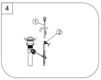
4. Insert lift rod (1) into sink hole, through the linker hole. Tighten the lock nut (2).
