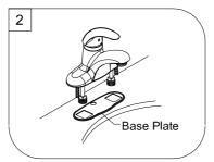
Shut off hot and cold water supply to faucet or turn off main water supply .
