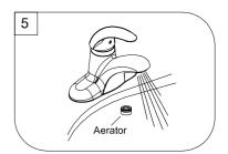
Remove AERATOR and turn faucet handle all the way on. Turn on hot and cold water supplies and flush water lines for one minute.
