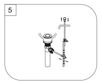
5. Move the linker along the ball rod, pull the lift rod knob up and down, move the linker at propriety location.
