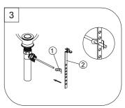
3. Install the spring clip (1) and linker (2) on the ball rod as shown.
