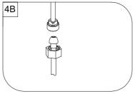
(B) Ball Nose Flexible Supplies: If you are using ball-nose flexible supplies to connect the faucet to water supply lines: Slip coupling nut behind ball-nose of flexible supplytube. Ball nose coupling will go partially into IPS shank or fitting. Tighten coupling nut (DO NOT OVER TIGHTEN).Install opposite end according to manufacturer's instructions for both tubes.
