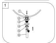
1-1. Remove flange (1), rubber washer (2), rubber washer (3), steel washer (4) and mounting nut (5) from the pop-up assembly.
