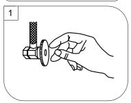
Shut off water supplies. Remove old faucet. Clean sink surface in preparation for new
