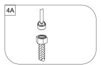
(A) Stainless Steel Braided Faucet Supply Tubes: This is the simplest of all installations. If you are using stainless steel braided faucet supply tubes, this faucet requires one end of the supply tube to have a 1/2" female IPS connection. The other end of this supply tube must match the thread on the water supply fittings or shut off valve under your sink. Once you have identified the required tube, carefully follow themanufacturer's installations instructions for each tube
