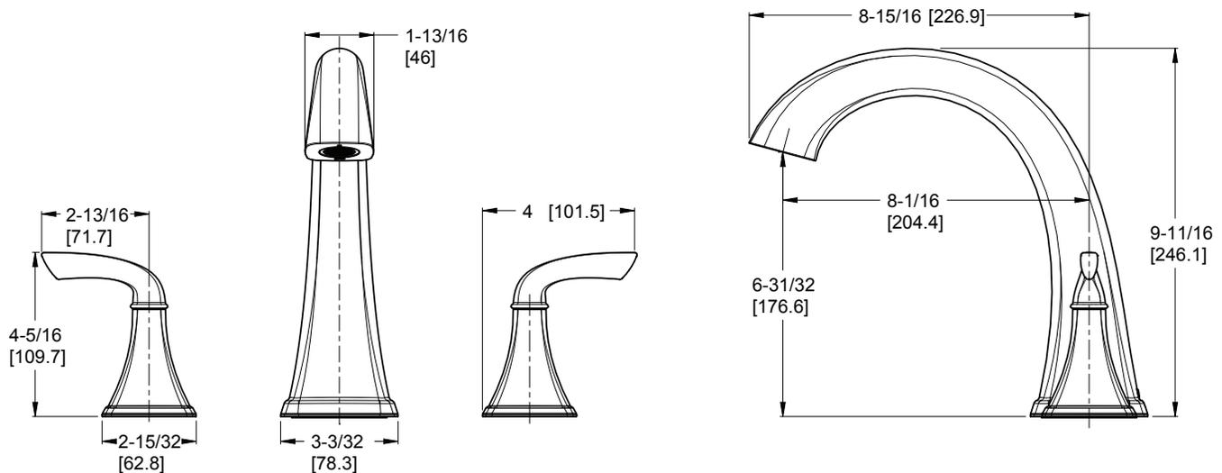
Ø1 Min to Ø1-1/2 Max. Deck Hole Openings
