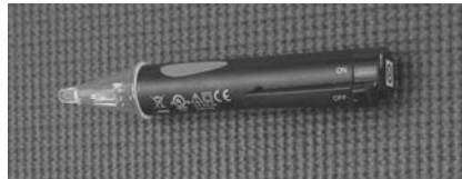
Figure 26 - Use a non-contact circuit tester to check for electrical power.
