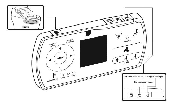
\*\*Press and hold "FLUSH" button marked with the water drop on the top left of the remote control to activate full flushing.
