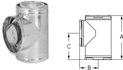
Use for through-the-wall chimney installations. The tee clean-out cap is removable for easy chimney cleaning or inspection. Wall Straps, a Wall Thimble, and a Tee Support must be installed with the Tee as directed. Tees have 1" insulating blanket. Ventilation air for chimney must be drawn from outdoors. (See installation instructions.)
