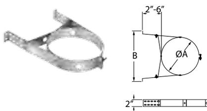
Use in interior or exterior installations to support and to stabilize the chimney while assuring a 2" clearance. Wall straps are required every 4' on exterior of building. Adjusts 2"-6" from wall.
