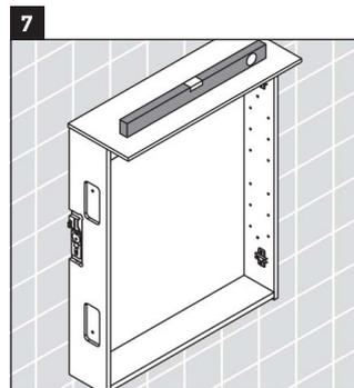
Check the cabinet is leveled and security attached to the wall.
