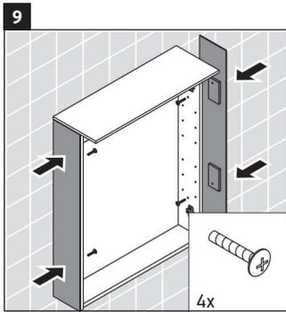
Attach side fronts with four supplied screws.
