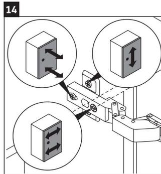
The top screw will adjust up and down. Back screw will adjust closer and further from the mirror cabinet and front screw will adjust left and right.
