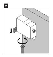
Using the screwdriver adjust the vanity mounting hinge system counter-clockwise.
