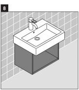
Slide the vanity under the washbasin. Tighten mounting bolts with a wrench until the washbasin is stable.
