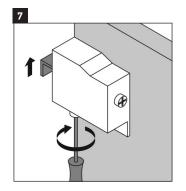
Using the screwdriver adjust the vanity mounting hinge system clockwise.
