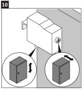
Screw two set screws until desired leveling of the vanity has been reached.
