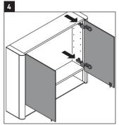
Remove the mirror fronts of the cabinet by unlatching each hinge.
