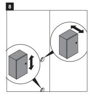
Check the scews which allow adjustments of the unit. The top screw will adjust front to back and the bottom screw will adjust up and down. Make adjustment to the level as needed.
