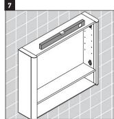
Check the cabinet is leveled and securely attachted to the wall.
