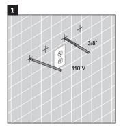
Reference the cabinet specification to establish the position of mounting bolts, mark the holes to be drilled for the anchors.
