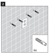
Drill the anchor holes that have been marked. Insert plastic anchors into the holes.
