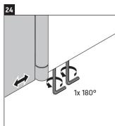
Using allen wrench tighten the bottom screws counterclockwise one turn 180 degree.
