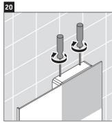
Using a screwdriver tighten the screws counter-clockwise.
