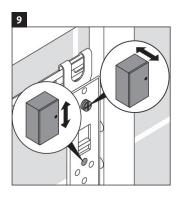
The top screw will adjust closer and further, from the mirror and lower screw will adjust up and down.
