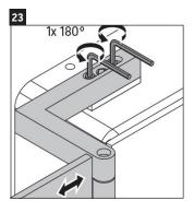
Using allen wrench, tighten the top screws clockwise one turn 180 degree.
