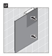
Push the mirror and attach to the mirror backing.
