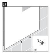
Attach mirror front to mirror backing with two bottom supplied screws.
