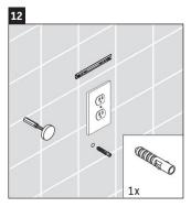
The plastic anchor provided is for concrete wall applications.
