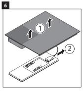
Lift the mirror up and slide the mirror backing.
