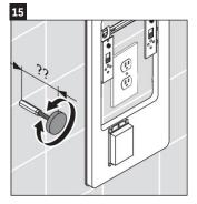
Adjust the length of the door stop by screwing it either, clockwise or counterclockwise.
