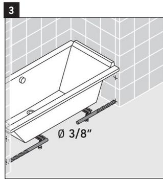
Using 3/8" drill bit, drill the anchor holes that have been marked.
