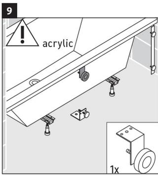
Attach one acrylic L-bracket to the tub.
