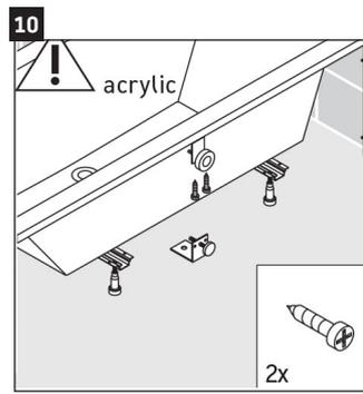
Screw the acrylic L-bracket to the tub using two supplied screws.
