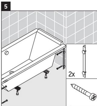
Screw the bracket(s) to the wall at the specified locations. For wood stud walls, bolts should be screwed into the wood backing.
