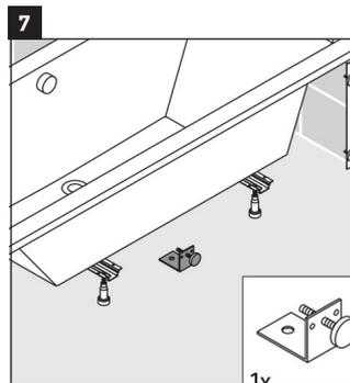
Install one L-bracket on the floor.
