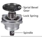
Lock Spring that joins Spindle and Sprial Bevel Gear protects the gears by absorbing shock casued accidental wheel lock during operation, ensuring longer tool life.
