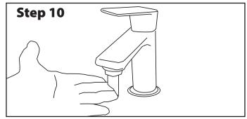
Check hot water at the fixture for desired temperature. If hot water temperature is not satisfactory, refer to the Troubleshooting checklist section.
