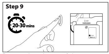
To test manual starter button, wait for hot water temperature to cool below 100°F (approx. 20-30 minutes). Push start button. The TacoGenie should run for a short time and shut off automatically.
