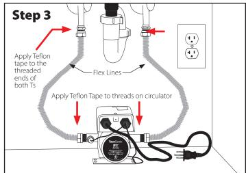
Apply teflon tape to threaded ends. Connect the flex lines to the tees, and to the TacoGenie Circulator.
