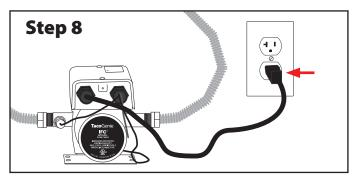
Plug in the TacoGenie. The pump will start automatically the first time only and run until a rise in temperature is detected by the thermal sensor. Pump will automatically shut off. Pump will be disabled when senses water temperature above 100°F.
