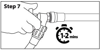
Check for leaks, flush system for 1-2 minutes.
