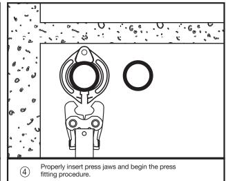
Procedure for laying the XL (copper and stainless) press ring around the XL (copper and stainless) Viega ProPress fitting with minimum space requirements.
