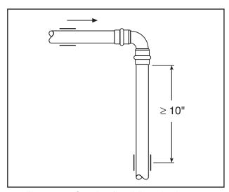
Figure 3.10 Spacing for sliding pipe hanger
