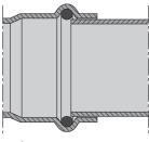
All Viega ProPress fittings are designed with cylindrical pipe guides to keep the pipe straight and protect the sealing element during assembly.
