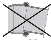
Fittings that do not have cylindrical pipe guides risk making an unsecure connection. Without the pipe guides, installers can possibly damage the sealing element.
