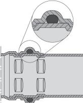
Viega fittings are pressed before, after and on top of the sealing element in a single step, which creates a permanent connection that is secure and guaranteed to last.
