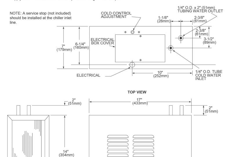
NOTE: It is important to insure proper ventilation. If this remote chiller is physically placed against barrier or in enclosure of any kind, 4" (102mm) air space must be allowed on all sides.
