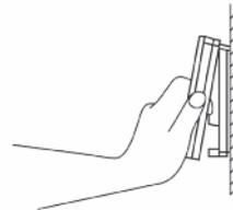
Locate wire terminals connector on rear of Tether Controller panel. Carefully connect wire to controller connector. Verify connector is secure, not loose and no external force on wires affects the connections at the terminals. Push extra cable into wall and secure controller panel to backplate mounted on the wall.
