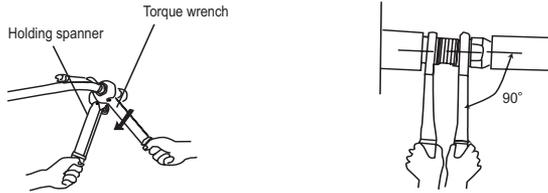
7. Carefully tighten flare nuts to correct torque level referring to the Torque Table below.
