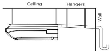
**NOTE:** Insulate condensate hose and/or pipes to prevent sweating which may cause water stains or wall damage.
