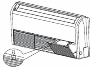
2. Locate and remove the screw securing right side panel. Remove right side panel from indoor unit by sliding it up and off as shown in the figure right.
