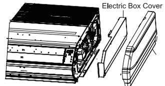
**NOTE:** Record wire colors and terminal references for uses with Outdoor Unit wire connections.
