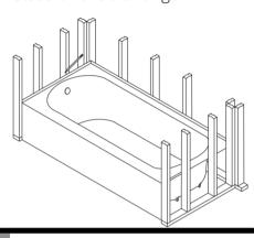
Remove the tub and install the drain. Predrill holes on the tile flange at the marked location of the studs.
