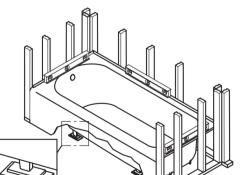
Secure the tub to the wall with galvanized screws. Screw into the predrilled holes. Put weight in the middle of the tub until the mortar sets.
