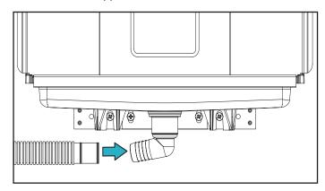
9. Route the drain hose through the filter box and attach the other end to the p-trap drain adapter using a hose clamp. The drain adapter is designed to be glued into a 1-1/4 inch PVC pipe.
