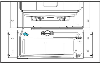
Connect the 1/4 inch water line from the water dispenser to the filter housing.
