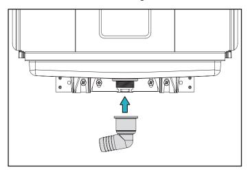
8. Attach one end of the 3/4 inch flexible drain hose to the 3/4 inch barbed drain adapter connection using the supplied hose clamp. The supplied flexible drain is 13 inches long. If a longer drain hose is required, it must be installer-supplied.
