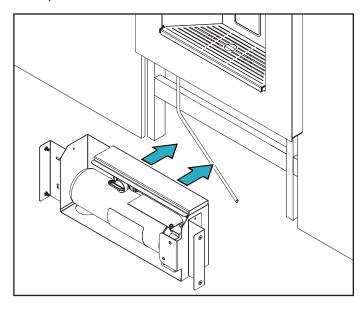
**Note:** Some side-to-side and up-and-down movement of the housing is capable to accurately align the filter unit with the water dispenser.
