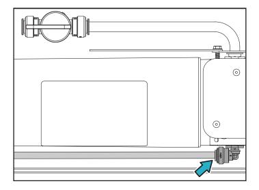
b. If the filter is installed in a remote location, attach an installer supplied length of 1/4 inch tubing to the 1/4 inch tubing from the water dispenser using a union coupling. The type of 1/4 inch tubing, copper or plastic, should meet all local regulations and building codes.
