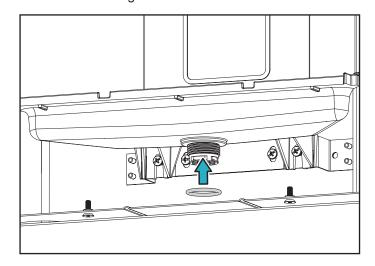
7. Thread the strainer into the drain adapter. Tighten the connection to create a watertight seal.
