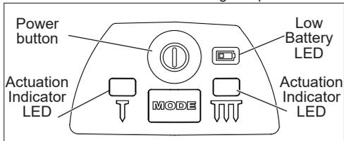
4. Press and hold the MODE button to toggle between single sequential actuation mode and contact (bump) actuation mode.
