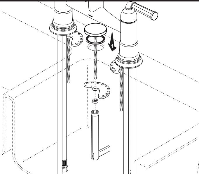
Insert body assembly through selected hole in sink. Secure assembly with bracket and nut. Use supplied wrench to tighten nut.
