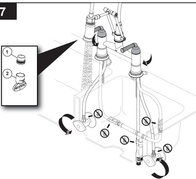
Remove aerator (1) using wrench (2) and turn faucet handles all the way on. Turn on hot and cold water supplies and flush water lines for one minute. **Important:** This flushes away any debris that could cause damage to internal parts. Reinstall aerator. Check all connections for leaks.
