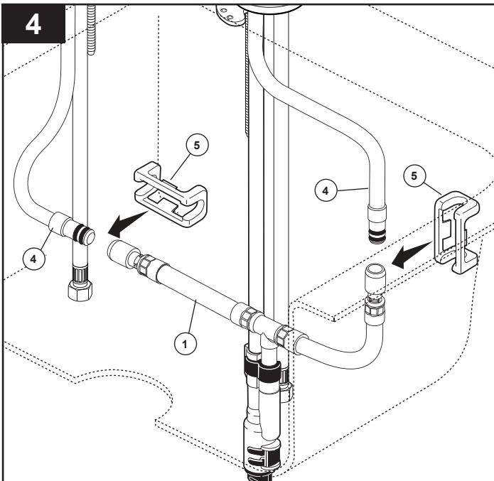
Insert ends of pex hoses (4) into ends of "tee" hose harness (1). Attach clips (5) over hoses. Pull hoses moderately to ensure connection is secure.
