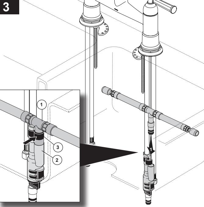
Slide "tee" hose harness (1) into top of diverter (2) and secure with clip (3). Pull moderately on tube to ensure connection has been made.
