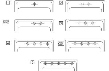
**Hole Drilling Configurations** 1-1/2" (32mm) Diameter Faucet Holes on 4" (102mm) Centers
