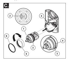
Rotate cartridge (1) so the words "HOT SIDE" (2) appear on the left. Insert cartridge assembly into rough-in body. Make sure the key (3) on the valve cartridge is fully engaged with the slot in the brass body (4). Insert bonnet nut (5) over the cartridge and thread onto the body. Hand tighten securely, slide o-ring (6) over bonnet and cartridge. A light coating of plumbers grease applied to o-rings may aid in assembly.
