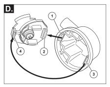
Snap temperature control cover over temperature control knob by first aligning smaller tab (1) on cover with receiving slot (2) on temperature knob. Swing larger tab (3) to engage with snap feature (4). Note: If dis-assembly is required, reverse this motion, disengaging larger tab (3) from snap feature (4) first.
