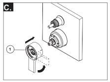
Install volume control handle (1) with lever pointing down, then turn to the on position. DO NOT SECURE WITH SCREW.
