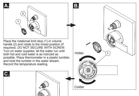
Secure temperature control knob (1) with screw (2). See next step (D) for securing temperature control cover (3).
