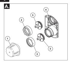
**Turn off water supplies.** Remove cover (1), bonnet nuts (2) and test caps (3) from the rough-in body (4).
