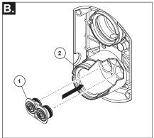
Insert adapter assembly (1) into rough-in body (2). Make sure the adapter assembly is correctly positioned and is pressed all the way down inside rough-in body.
