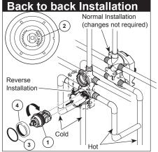
For the exceptions of back to back or reverse installations (hot on right and cold on left) only: Rotate valve cartridge (1) so "HOT SIDE" (2) appears on the right.
