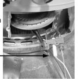
Step 9. Thoroughly inspect the burner surface area and burner port area and remove any loose debris.
