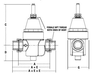
ABOVE VALVE SHOWN WITH SINGLE NPT UNION CONNECTION ON INLET VALVES MAY BE ORDERED WITH 0.1.0R 2 UNION CONNECTIONS USING ANY COMBINATION OF NPT. SOLDER, PEX OR CPVC CONNECTIONS REQUIRED "F" DIMENSIONS ARE APPROXIMATE FNGAGEMENT LENGTHS.
