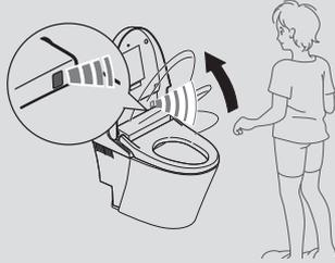
The upper body sensor detects changes in heat (person's movement).
