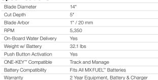
Kit Includes: MX FUEL™ 14" Cut-Off Saw. (1) MX FUEL™ REDLITHIUM™ XC406 Battery Pack, MX FUEL™ Charger, Wrench, Hex Key, Quick Connect, Contractor Bag
