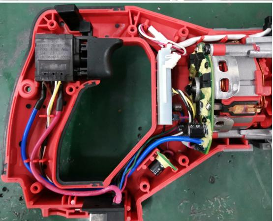
As an aid to reassembly, take notice of wire routings and position in wire guides and traps while dismantling tool.
