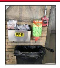
Hearing protection is used by all core trades to protect against hazardous jobsite noise. OSHA recommends that users not be exposed to a noise level greater than an average of 85 decibels over 8 hours\*.
