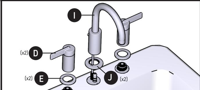
**WARNING:** Always turn water supply OFF before removing existing faucet or disassembling the valve. Open faucet handle to relieve water pressure and ensure that complete water shut-off has been accomplished.
