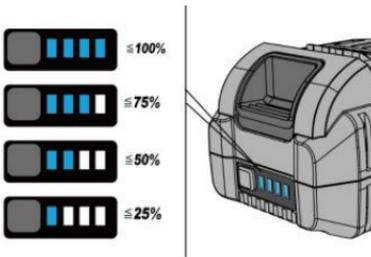
The indicator goes out after 3 seconds. If the LED lights red, the battery must be recharged. If the LED not lights up after the button is pressed, the battery is faulty and must be replaced.
