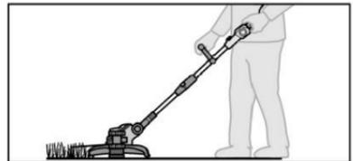
the ground. When clearance cutting, guide the trimmer in a semi-circle in front of your body.
