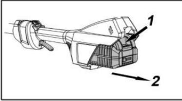
**CAUTION:** *Protect the battery contacts when the battery is not being used. Loose metal parts may short-circuit the contact. **Explosion and fire hazard!***
