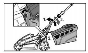
Adjusting the Cutting Height The cutting height can be adjusted from 0.98" to 2.95".
