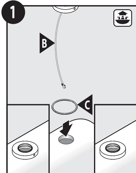
Install Escutcheon with Indicator Light (B) & O-Ring Gasket (C) on to deck.
