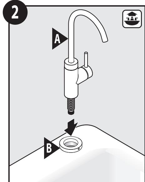
Install Faucet Body (A) thru Escutcheon (B) & hole in deck.
