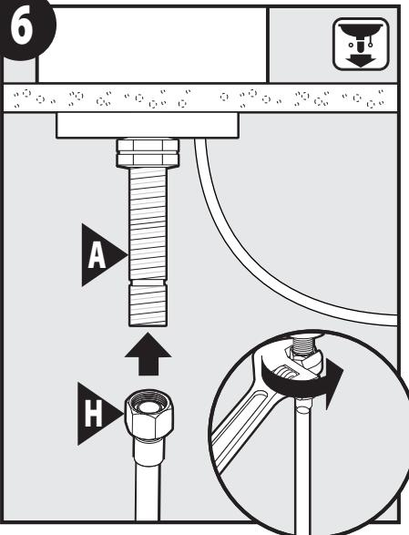
Connect Supply Line (H) (not included) to Faucet Body Shank (A). Tighten with wrench. **Note:** If using Filtration System (S5500), then this supply line will be Filter Outlet Hose (D) from INS10244.
