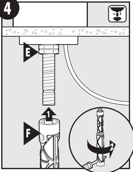
Tighten Mounting Nut (E) with Installation Tool (F).
