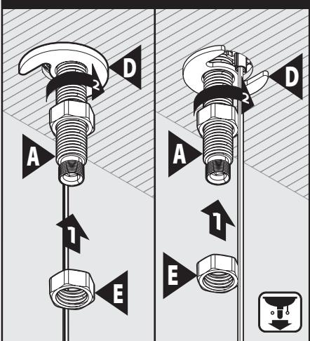
Install Mounting Washer (D) on Faucet Body Shank (A). Secure with Mounting Nut (E). Do not pinch wire with Mounting Washer (D). **Important:** thread light cable through open side of washer (D). Use care to make sure light cable is not pinched.
