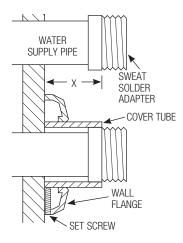
Tighten wall flange set screw with hex wrench supplied. **DO NOT** install vandal resistant stop cap at this time.
