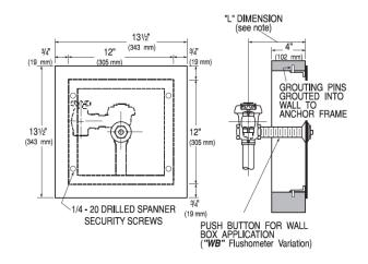
**NOTE:** "L" Dimension is the Wall Thickness (to the nearest whole inch) plus 2%". Specify "L" Dimension when ordering Flushometer.
