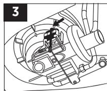
3 Unclip the battery from wire and replace with fresh battery.
