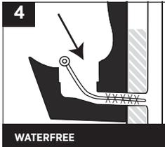
4 Scrub the housing and deep inside of the tail pipe with a long 1.5" diameter nylon brush.
