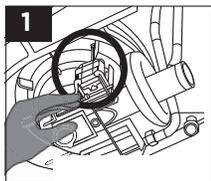
1 Reach underneath the urinal and locate the battery.
