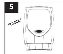
5 After 1 minute the unit will be ready for operation. Swipe hand within 2 inches of sensor and visually inspect that water flows into housing, ensure cartridge is out of housing for inspection.
