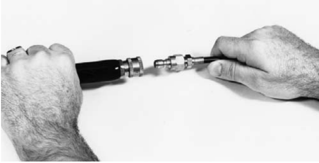
Figure 3 – Connect jetter hose to jetter
