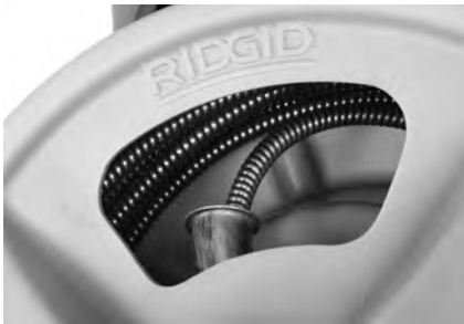
Figure 18 – Coil Cable Into Drum As Shown
