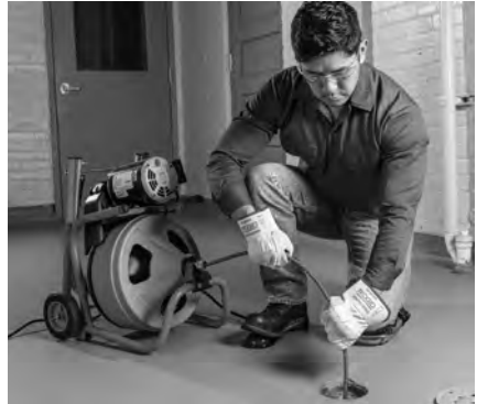
Figure 13 – In Operating Position, Manually Feeding Cable
