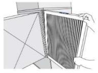
Central unit: slide filter into unit
