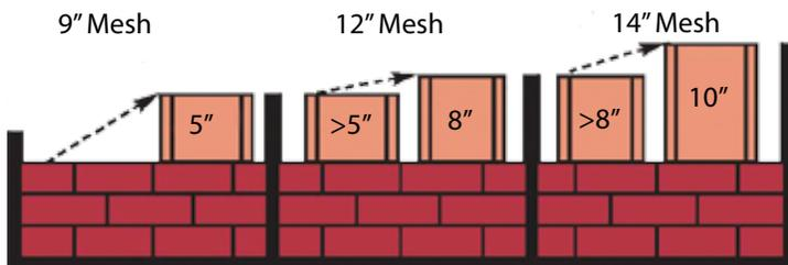
For Copper, standard 9" expanded metal mesh is used when flue tile height is 5" or less. If tile height is greater, refer to the chart.
