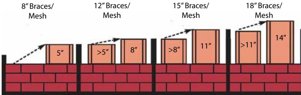
For Aluminum and Stainless Steel, standard 8" braces and expanded metal mesh are used when flue tile height is 6½" or less. If tile height is greater, refer to the chart.
