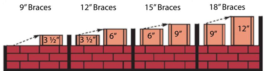
Standard 9" braces and expanded metal mesh are used when flue tile height is 3½" or less. If tile height is greater, refer to the chart.
