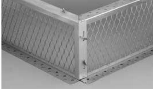
Easy to assemble with tab and slot corner design. Hood attaches to base with weld bolts and nuts; no chance of stripping out threaded holes. Hinged mounting flanges available on Stainless Steel and Copper models.
