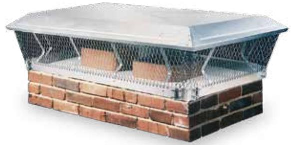
The hood overhangs masonry approximately 3" on both sides and ends. The cover attaches securely to the chimney with a 2¼" draw band. Four adjustable corner clamps provide ample flexibility for proper fit.
