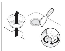
Remove flange old flange from sink. Remove plumber's putty from sink with putty knife.
