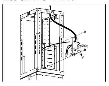
Remove wiring cover and connect house wiring to hood wiring
