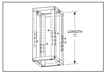
Determine length "L" of frame assembly based upon desired installation height (see chart below.) To adjust frame assembly height, remove (8) screws, slide upper frame assembly to required height, replace screws and tighten securely.
