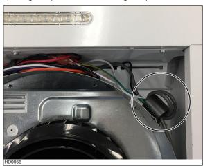
② Open the provided connection box. Using long nose pliers, break away 2 cable entry notches on the lid (one per side).
