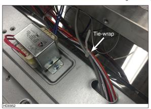
① Close the control access panel and reinstall the blower by reversing steps ⑥ to ③ on first page. Run the ADA cable section through the provided ferrite, making 2 loops. The ferrite must be as close as possible to the access panel.
