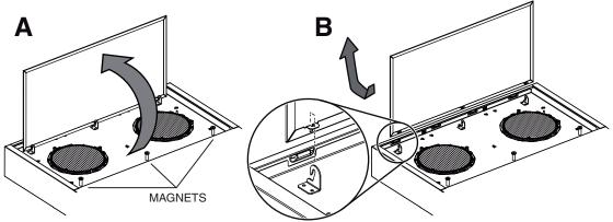
Using a 11/32" nutdriver or socket, remove both lock nuts retaining the flange of the cover plate to the inner back of hood (see insets). Remove the cover plate retaining screws (9 screws), then set the blowers cover along with its screws and nuts aside.
