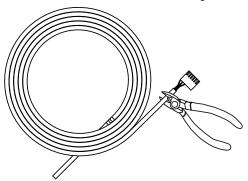
Sun one end of the ADA cable through the range hood wire clamp, along with the power cable, giving enough length to make the connection inside the box. Tighten the wire clamp, then strip the end of the 3 wires from provided ADA cable.
