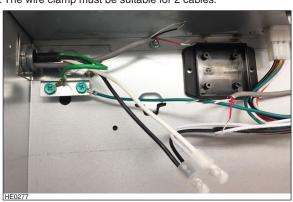
Using small UL approved wire nuts (suitable for 22 AWG wires), connect wires as follow: WHITE wire with WHITE wire, BLACK wire with BLACK wire and RED wire with RED wire.
