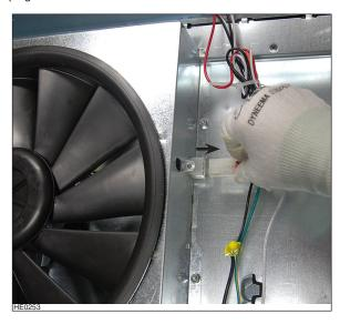
● Using a 11/32" socket, remove the 6 nuts retaining the blower chamber to the hood assembly (2 nuts on inner back and 2 other nuts per sides), then use a Phillips no. 2 screwdriver to remove both front corner screws. See picture below for nuts and screws locations. Pull the blower chamber out of the hood assembly and set it aside with its retaining screws and nuts.
