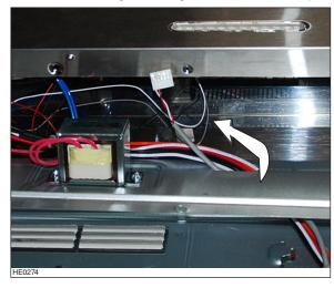
S Connect the ADA cable connector to the 6-pin connector on control board (circled on picture below).
