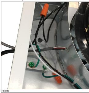
Strip the end of the 3 wires from GREY cable (the one with ferrite), then using small UL approved wire nuts (suitable for 22 AWG wires), connect these wires with ADA cable wires. Connect as follow: WHITE wire with WHITE wire, BLACK wire with BLACK wire and RED wire with RED wire.
