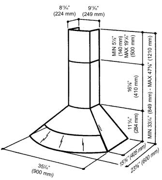
Mount range hood so bottom of hood is 24" to 30" (610 mm to 762 mm) above cooking surface.
