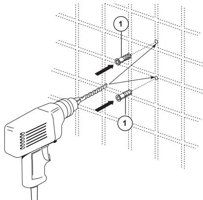
**NOTE: If possible, it is best to mount your accessory into a wall stud. Try to locate a wall stud with a stud finder or by tapping on the wall.**
