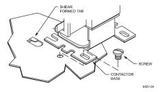
Fig. 1. Typical contactor mounting.
