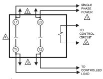
POWER SUPPLY. PROVIDE OVERLOAD PROTECTION AND DISCONNECT MEANS AS REQUIRED.
