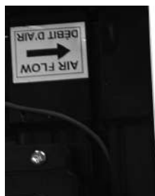
Fig. 18: Make sure that the arrows on the filter point in the same direction as the arrow on the enhancement module. This will be in the same direction as airflow.
