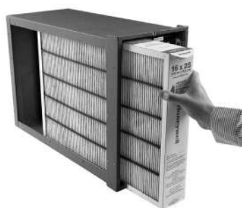
Fig. 18: Make sure that the arrows on the filter point in the same direction as the arrow on the enhancement module. This will be in the same direction as airflow.
