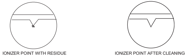
Fig. 19. Removal of deposits from ionization points.
