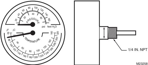
**Application:** Pressure/temperature gauge with relief set point indicator
