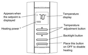
\* The thermostat displays the percentage of heater duty cycle required to maintain the desired temperature. For example, if the heater is activated 40 percent of the time, \$\int\_{\mathfrak{1}}\$ is displayed.
