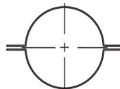
Use to position the Vertical Termination for Commercial Systems (VTM's) to the variable pitch roof flashing. The clamp is upsized one diameter to fit around the black metal outer pipe. The support clamp rests in notched groove of variable pitch roof flashing.
