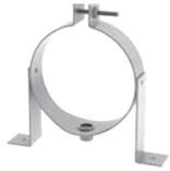
Use to support single-wall and concentric offsets and pipe used in vertical rise or horizontal runs as per installation instructions. Wall Strap legs can be rotated up to 360° for versatility. Accepts standard 3/8" all-thread. Available in galvanized or stainless steel metals. Note: Vent pipe must be supported at least every 10 feet (3m) vertically. Horizontal or sloped sections of vent pipe require a wall strap on each pipe section.
