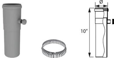
Use for combustion analysis testing without drilling holes into the vent system. Port cap is threaded for easy removal. Install immediately above the appliance. Includes 1 Locking Clamp.
