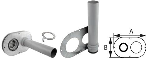
Use to adapt PolyPro to the IpeX 636 low profile termination. Kit includes 14" pipe welded to an adapter and metal backing plate. Check with appliance manufacturer for approval. (Outer IPEX termination cap not included. Supplied by others.)
