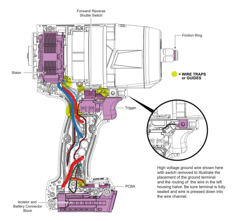
Be sure that all wires of the electronics assembly are routed as shown, being careful to push down completely into wire traps. Be sure that the trigger switch, PCBA, battery connector block, stator and shuttle switch are fully seated prior to installing the handle cover.
