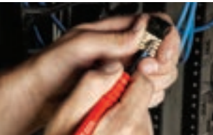
Wire Pick & Hook for Removing Errant Connections
